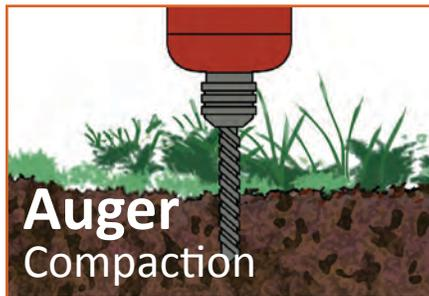
Use an 18" long x 5/8" diameter masonry drill bit with a hand drill to make targeted holes in compacted soils. Drill holes throughout the compacted area, and keep them at least 12" apart on center. Follow this hole-making with good compost or worm castings, and thoroughly water in everything.
