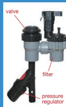
Irrigation valves are designed to work within a certain pressure range (pounds per square inch or psi) and flow range (gallons per minute or GPM). If you redesign your system and use low flow irrigation, the flow through the valve may be so low that your existing valve will not operate effectively and may get stuck in the "open" position, wasting water. If you have flow lower than 5 GPM per valve, check your valve specifications for flow range to determine whether or not to replace your valves.
